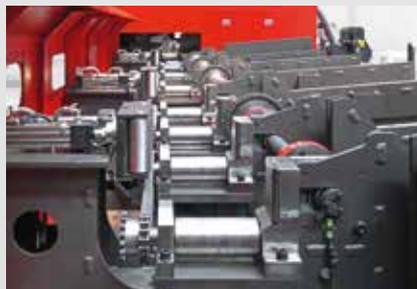
**Loading magazine with 10,000 kg capacity (CMB 230)**
