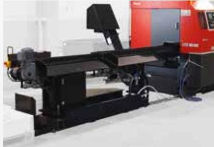
**Slat conveyor with sorting channels**
