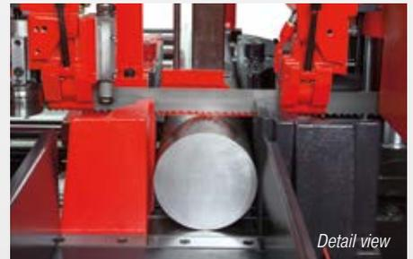
The use of a SMARTCUT 41 mm band saw blade with only 0.9 mm blade thickness specially developed for this machine type, reduces the waste by 25 %, which is particularly advantageous with respect to the efficiency during sawing of expensive materials. This makes the robust, column-guided AMADA PCSAW 330 particularly interesting for large series.
