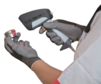
Obtain tooling information from bar-code
