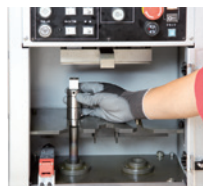
Setting the tool on the measuring unit
